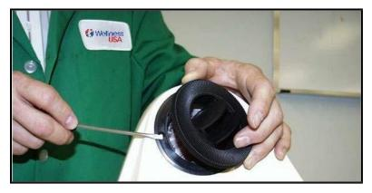
Figure 7.16.1 Removing Face Air Vent(s).
