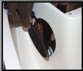
Figure 7.3.2 Removing Hinge Plate.
