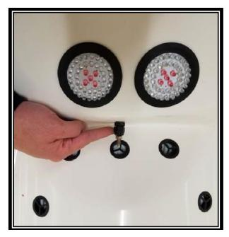
Figure 7.22.1 Heat Sensor Location inside the Hood.
