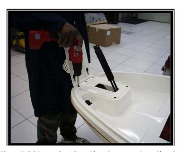
Figure 7.6.2 Removing Hinge Plate Screws on Base Chassis.
