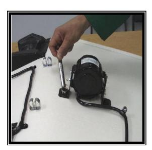
**Figure 7.9.4**Removing Flange Bolt Attaching Motors.
