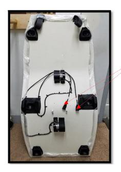
Vibration motor controller connections
