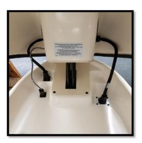
Figure 7.1.1 Releasing Electrical Connectors.
