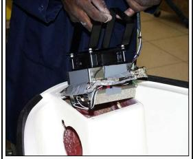
Figure 7.3.4 Removing Heater Harness.
