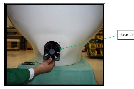
Figure 7.17.1 Inserting/Removing Face Fan Assembly.
